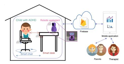
Fig. 1. Schematic of the SmartHome environment designed for pervasive occupational therapy for children with ADHD. This depiction shows the placement of various sensor devices and the robotic assistant within the house. These tools capture detailed information about the workspace, which is then relayed to Firebase for processing. The processed data can subsequently be accessed and visualized by therapists and parents via the mobile application developed in the course of this research.
