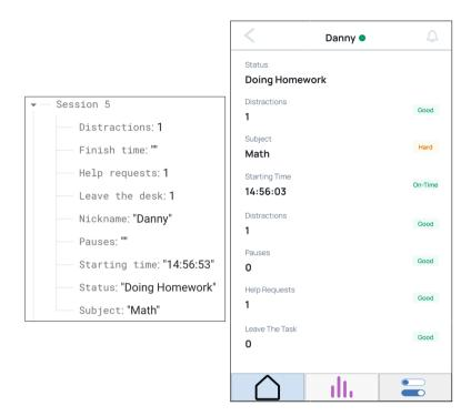
**Fig. 3.** (Left) Depiction of real-time data acquisition as represented within the Firebase real-time database, demonstrating the process of sensor reading collection. (Right) Visualization of the processed information within the mobile application, structured for easy comprehension and practical use by therapists and parents.
