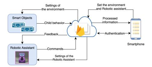
Fig. 2. Illustration of the interaction mechanism among the smart objects, the robotic assistant, and the mobile application, facilitated via Firebase. This diagram underscores the communication flow and data exchange among these entities in the context of the SmartHome environment.
